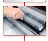
**Step 4:** Fold down the cutter so that the film is held in place and then pull the cutter knife across the film
