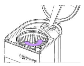
Press the filter holder down and turn the handle to position "close".
