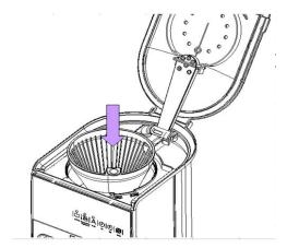
Put the filter holder in the device so that the handle is at position "open".
